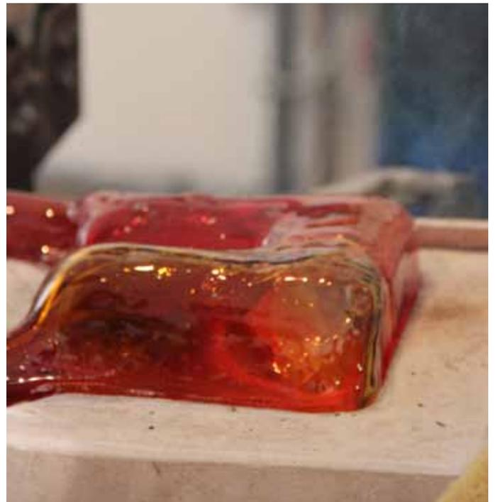
**Tandem Alan-Fabien** blowing the glass at the same time and the glass blown into the plaster mold
